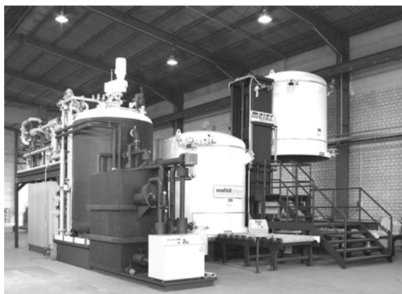
Figure 1: VPI equipment for global impregnation of medium-sized high voltage stators (Von Roll Isola – Meier GmbH).
