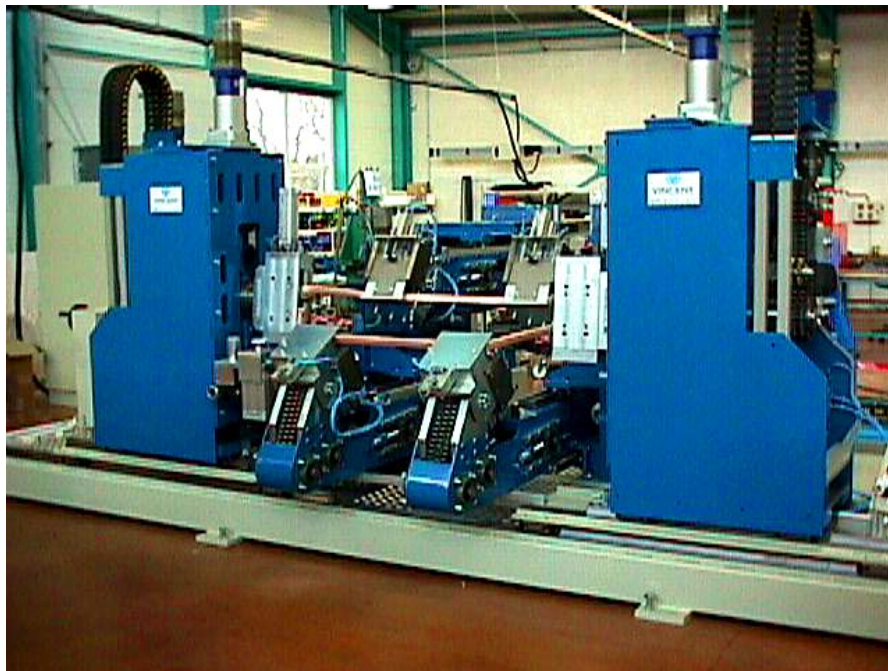
Figure 1: Coil forming machine for fully insulated flat coils
