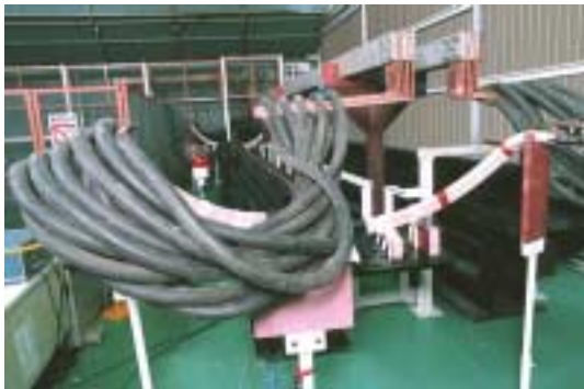
Fig.8 Thermal cycling test of HTC insulation coils
