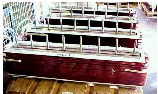
Figure 6 Pole coils produced with Thermibond ® M
