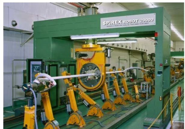
Figure 5: Application test of HTC mica tape on full size Roebel bars
