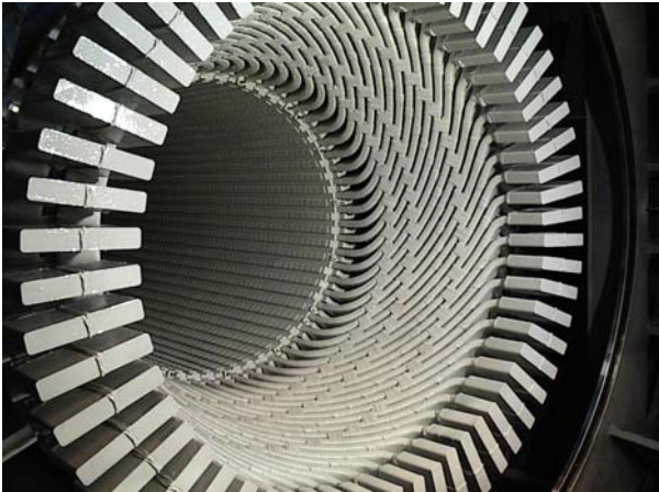
Figure 9: Stator of a 250 MVA turbo generator equipped with the HTC insulating system
